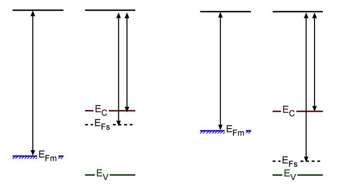
(2) Draw a diagram of TWO ways to make an ohmic contact on a n-type semiconductor, and then explain to the Prof. how each works.
